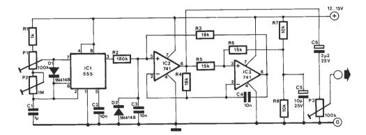
This circuit will simulate the sound of a bell or gong and may be used as a replacement for conventional bells in such applications as doorchimes, clocks etc.
