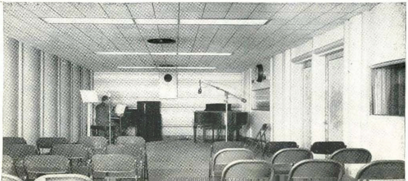
Fig. 3—This studio at WRRN is approximately 16 x 36 feet and can accommodate an audience of 100 people. Reference to Fig. 1 shows the relation of this studio to the associated control room and its convenient relation to the entrance lobby of the station.
