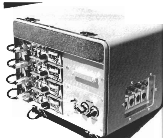
Four receiver "field pack" carrying case with: internal common battery supply, common headset monitor, input/output connectors for power and audio. Storage compartments are provided for transmitters and cables.
