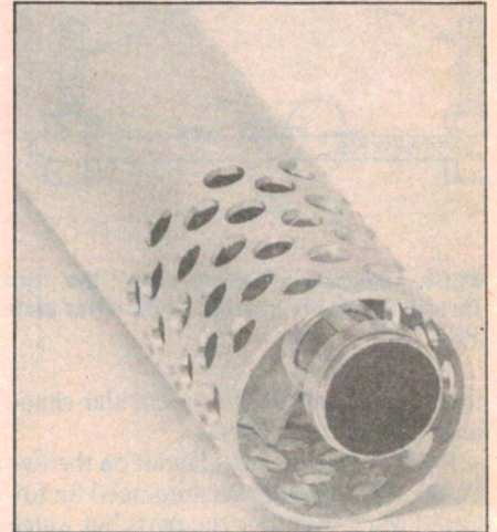
The "business" end of The Microphone. The electret insert is clearly visible.
