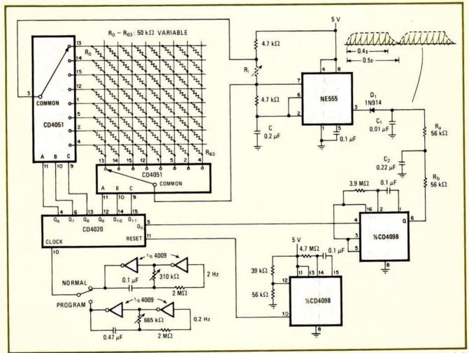
**Tuning up.** Music box/tone generator uses programmable resistor matrix to generate 64 tones in sequence, each for a 0.5-second period. Oscillator clocks 4051s, which in turn place each of 64 resistors in timing network of 555. Output of timer is shaped by a 4098 one-shot and suitable integrator network for click-free output during switching. Matrix can be programmed in 10 minutes if counter is available.
