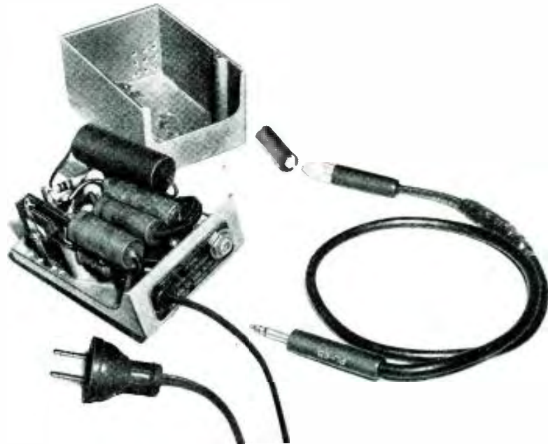
After wiring the switch, the fiber banana-plug strip is placed over contacts to insulate them.
