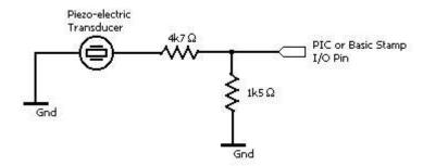
The circuit above illustrates the interface between a piezo transducer and a PIC data pin. When the transducer (or a surface to which the transducer is attatched) is struck, a voltage is generated which may be detected at the data pin. Suitable software would scan the data pin(s) and transmit a MIDI message when a high (1) logic state is detected.
