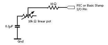
The Basic Stamp I POT command performs the above process and returns a scaled output value. See <u>Scot Edwards' Parallax assembler version of the POT command in *The PIC Source Book*</u> for an example of using the above circuit with a PIC chip.
