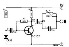
internal noise produced by the diode is amplified by the single stage preamplifier, consisting of T1 and its associated components, which is designed for high gain and low cost. T1 can be almost any silicon NPN transistor, a BC107 being used in the prototype.
