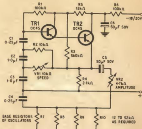
Fig. 7.2. Bridged-T vibrato sine wave oscillator
