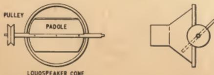
Fig. 7.5. Rotating paddle vibrato system
