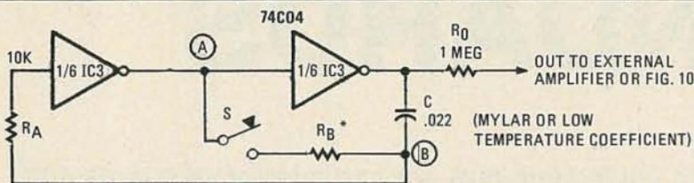
\*R<sub>B</sub> IS SHOWN IN MORE DETAIL IN FIG. 6 AS A SERIES OF 6 FIXED RESISTORS.
