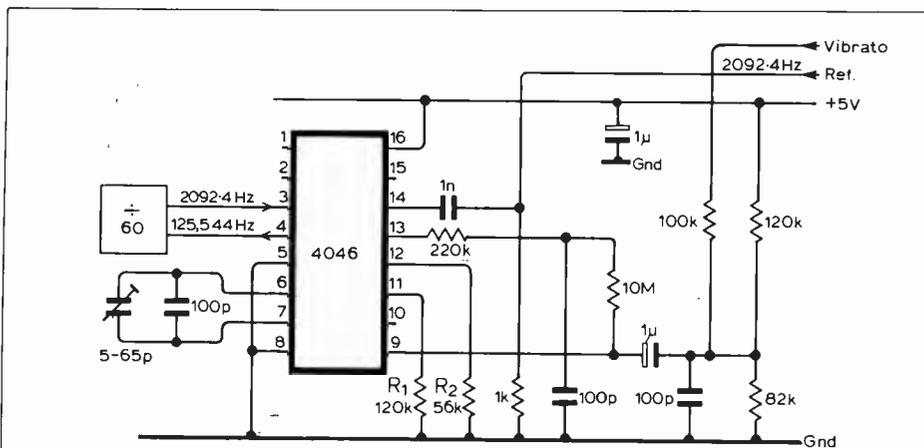
Fig. 10. Phase lock loop for C card. This circuit multiplies the reference frequency by 60.
