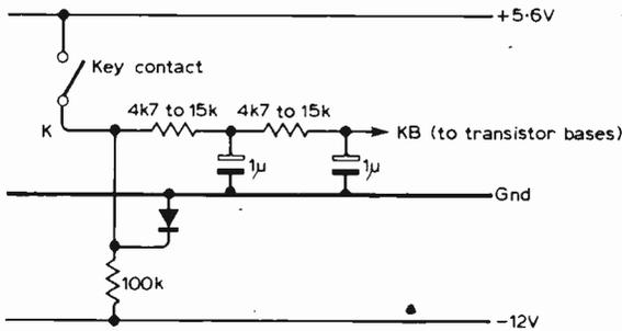
**Fig. 14. Keying circuit.** The double integrating network is used to control a d.c. output component by shaping the keying envelope.
