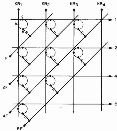
**Fig. 15. Portion of the three-way matrix.** This layout is roughly the same as the p.c.b. viewed from below.
