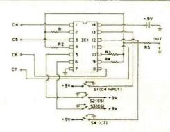
Music Maker" project. The voltage should not the combining via the switches. The switch exceed 9 volts at these inputs. The output will be marked "S1" will put the C4 input through to the a combination of the inputs, where you control output when it is switched to the down position.
