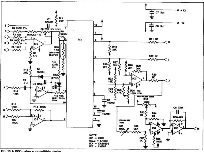
Fig. 13 A VCO using a monolithic device.
