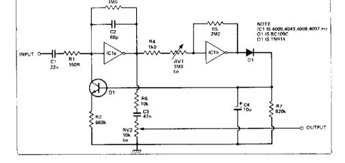
increase in proportion to the input level from the guitar. RV2 can be set to any desired level and when set high can easily overdrive the input stage of the guitar amplifier giving a tube-type of distortion.
