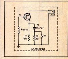
R1 (and an additional 5.1M resistor from the FET gate to ground) may be mounted in the cable jack.
