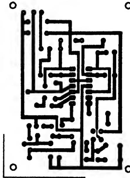
Fig. 6: Actual-size PCB pattern for the circuit.
