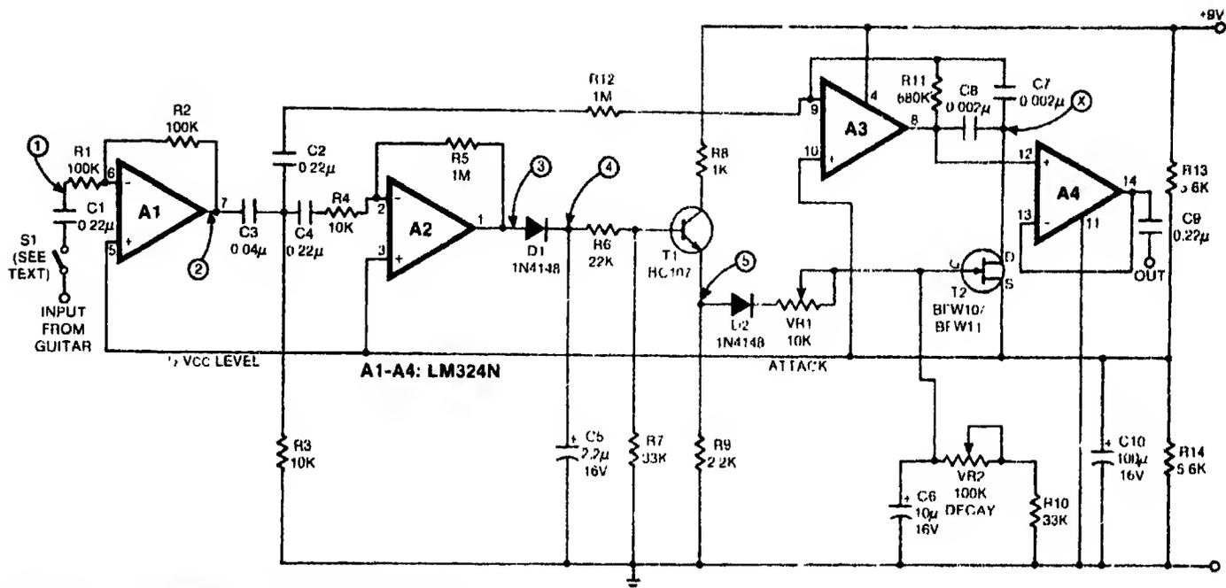
Fig. 2: Circuit diagram for the envelope follower.
