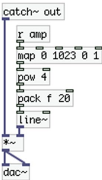
Figure 4-8. Contents of the audio_out subpatch
