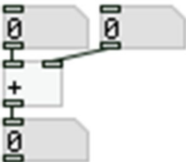
Figure 1-10. A control domain patch
