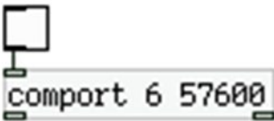
Figure 2-27. Simple patch to control an LED of the Arduino
