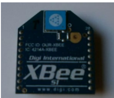
Figure 3-21. XBee series 1 with trace antenna
