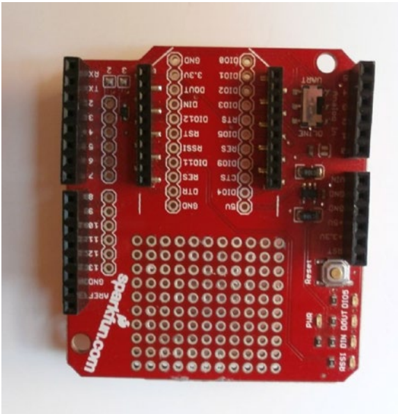
Figure 3-22. XBee Arduino shield
