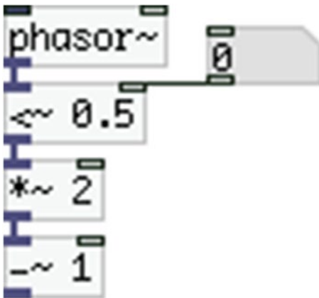
Figure 1-23. The square wave oscillator Pd patch
