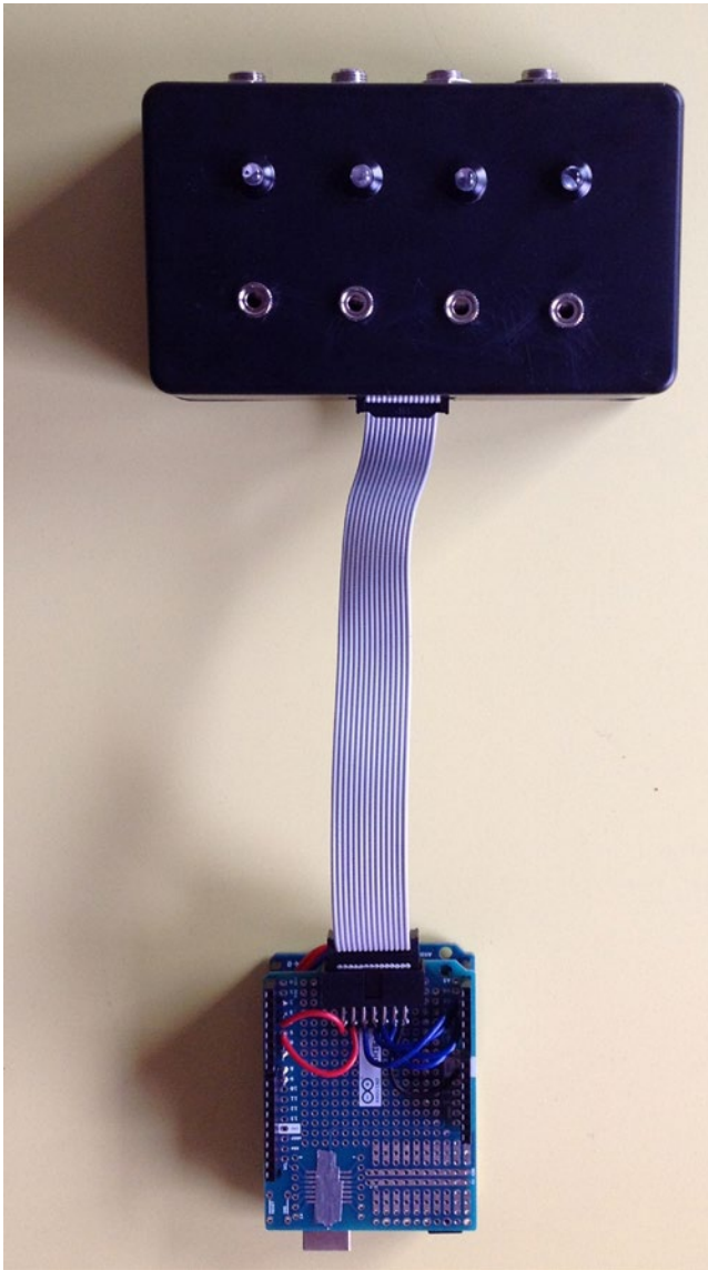
Figure 7-29. Connecting the circuit box to the Arduino
