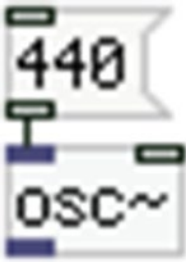
Figure 1-3. A message connected to an object
