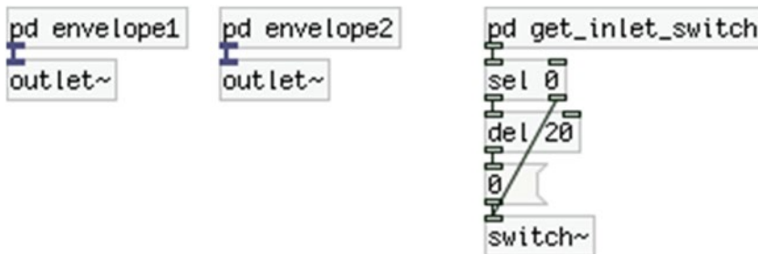
Figure 10-31. The envelope~ module abstraction
