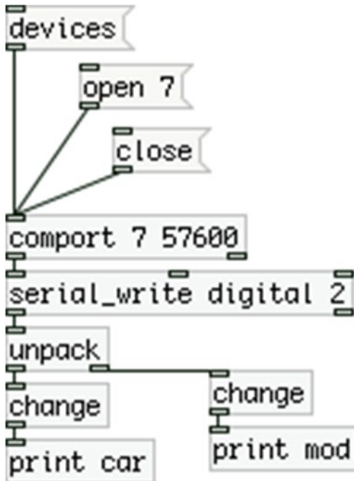
Figure 8-16. Pd patch to receive the waveform data from the Arduino
