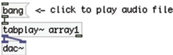
Figure 1-27. An audio file playback patch
