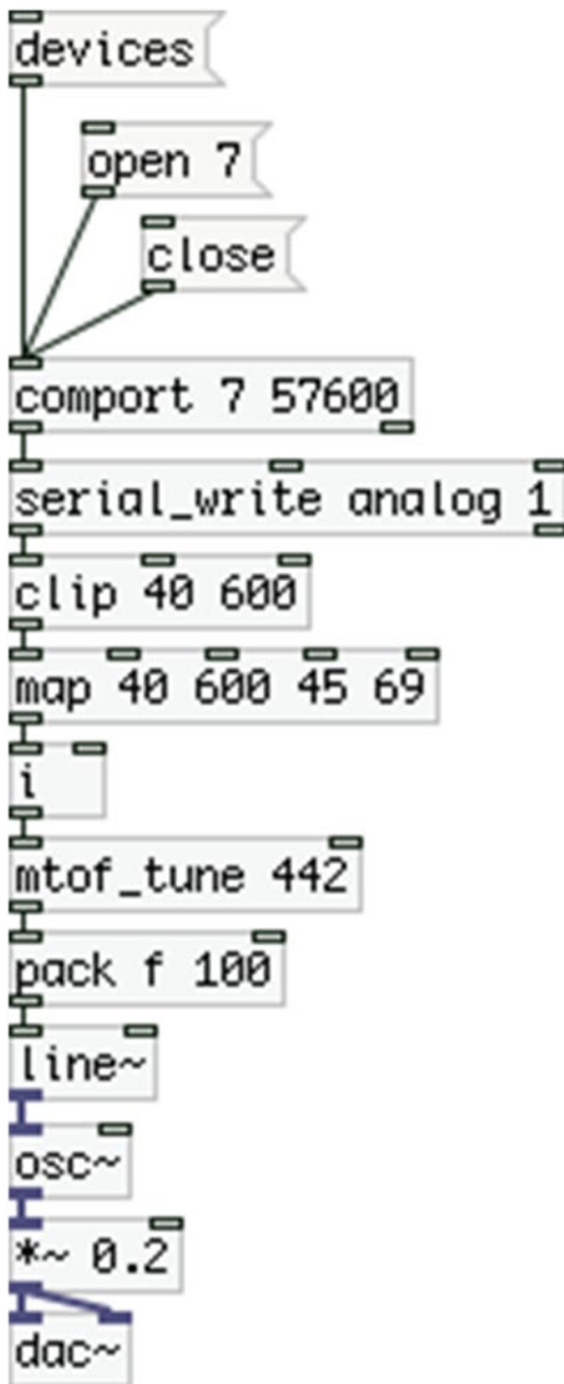
Figure 8-3. Pd patch receiving smoothed values from the infrared sensor
