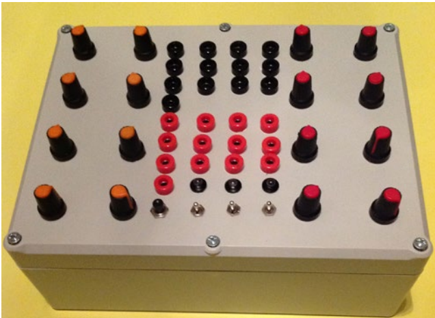
Figure 10-40. A patch-bay matrix synthesizer layout
