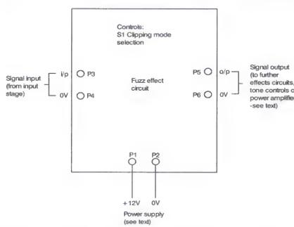
Fig 8 Fuzz effect circuit terminal connections
