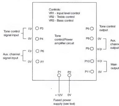
Fig 10 Tone control/power amplifier terminal connections
