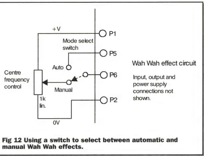
**Fig 12 Using a switch to select between automatic and manual Wah Wah effects.**
