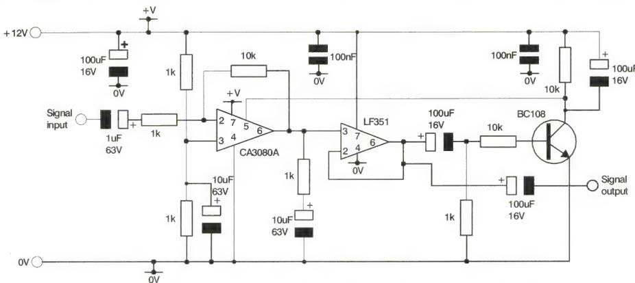
**Fig 11 Experimental limiting circuit**
