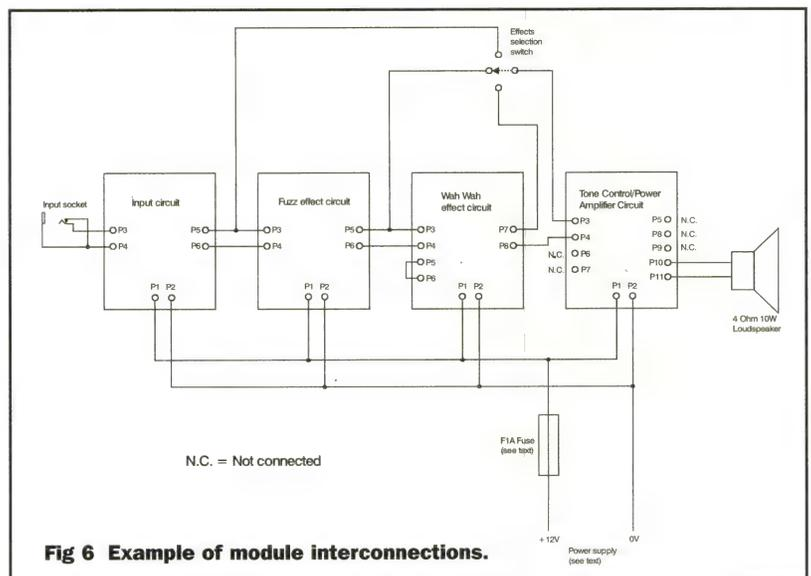
Fig 6 Example of module interconnections.
