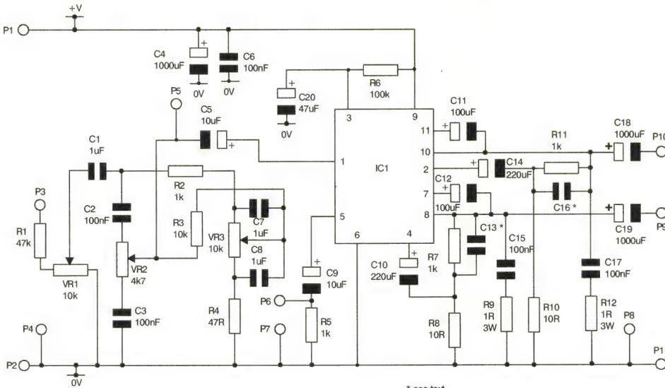
Fig 4 Tone control/power amplifier circuit diagram
