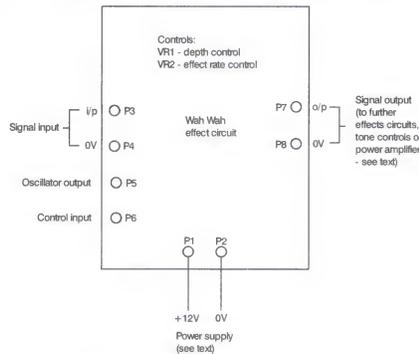
Fig 9 Wah Wah circuit terminal connections
