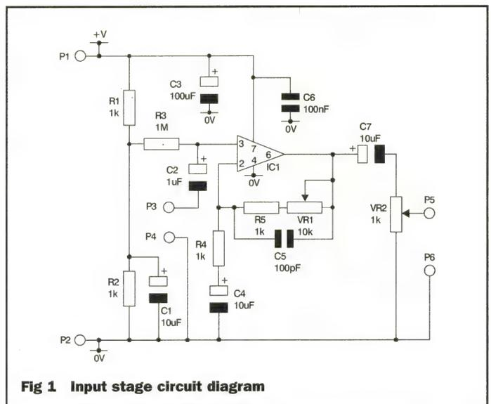
Fig 1 Input stage circuit diagram
