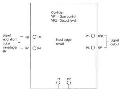
Fig 7 Input circuit terminal connections
