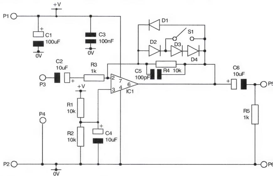
Fig 2 Fuzz effect stage circuit diagram
