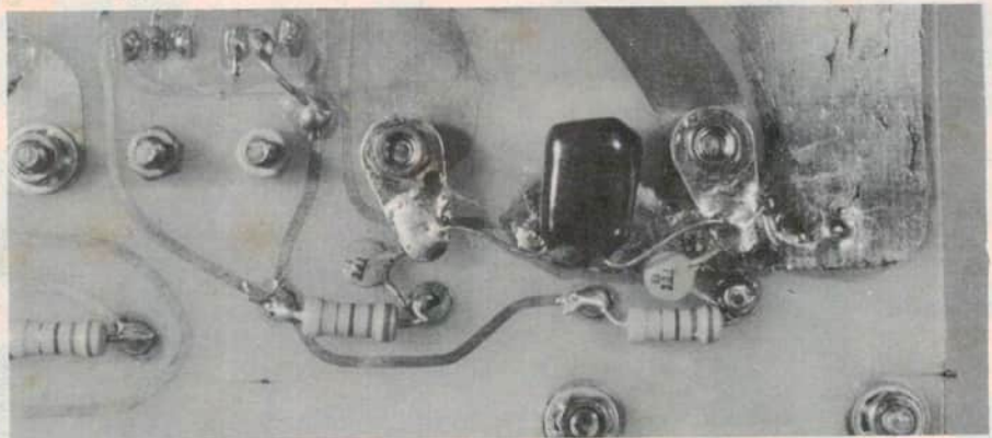
Compensation capacitors are required for the two 2SK134 output MOSFETs (Q8 and Q9) to equalise the input capacitances between the n-channel and p-channel output devices. They are mounted under the board as shown here. Solder lugs are placed on top of the mounting nuts and held with another nut each. C6 and C7 mount from these to the pads shown, while C7 mounts between them. Note the resistors mounted under the board also.
