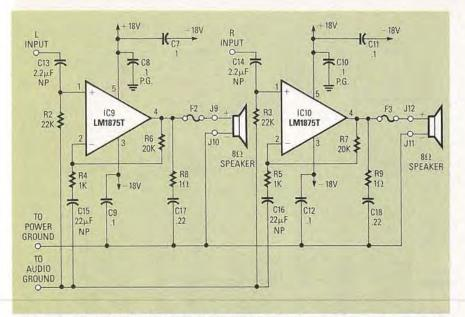
FIG. 6—THE SURROUND CHANNEL POWER AMPLIFIERS are designed around a pair of LM1875 monolithic power-amplifier IC's.
