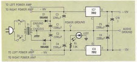
FIG. 7—THE POWER SUPPLY produces about ±18-volts unregulated DC.
