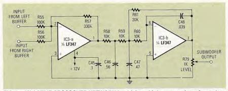
FIG. 3—AN ACTIVE CROSSOVER NETWORK for driving a high-power subwoofer system is made from IC3-a and IC3-b.
