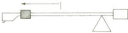
Fig. 3—An adjustable weight, able to be moved along the tonearm tube, can be positioned toward the pickup to increase arm mass.
