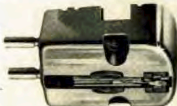
Fig. 4-2. The G. E. variable reluctance pickup. There are two gaps: when the iron in the stylus assembly is moved out of one gap it is simultaneously moved into the other.
