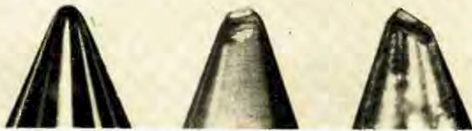
Fig. 4-6. One mil microgroove needles after 15 plays of a 12-inch Vinylite record, with 8 grams vertical tracking force. Left to right: diamond, sapphire, and osmium. (After Marcus).
