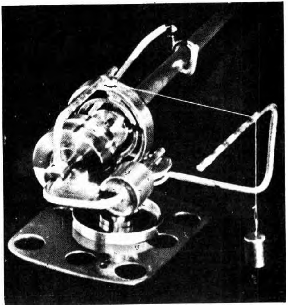
Rear view of mounting post and weighting arrangements for author's pickup arm.
