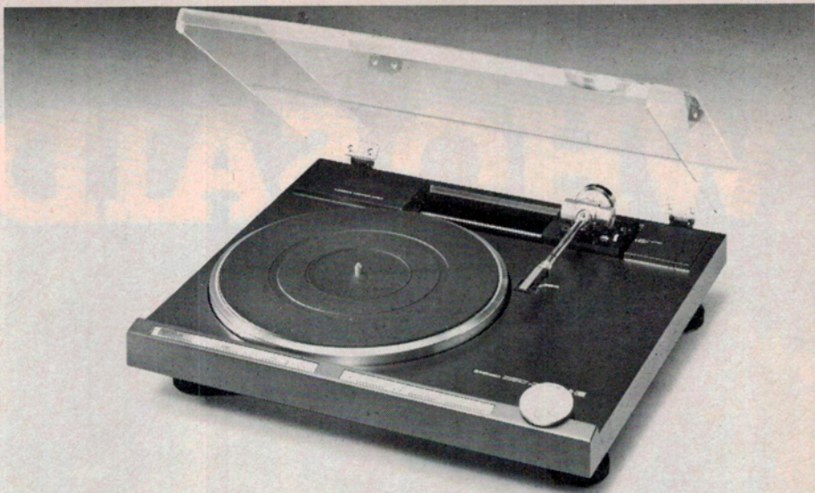
The Pioneer PL-L1000 features a tangential tracking tone arm driven by a unique linear motor system. It employs an optical tracking sensor to maintain the arm position to within 0.2° of deflection.
