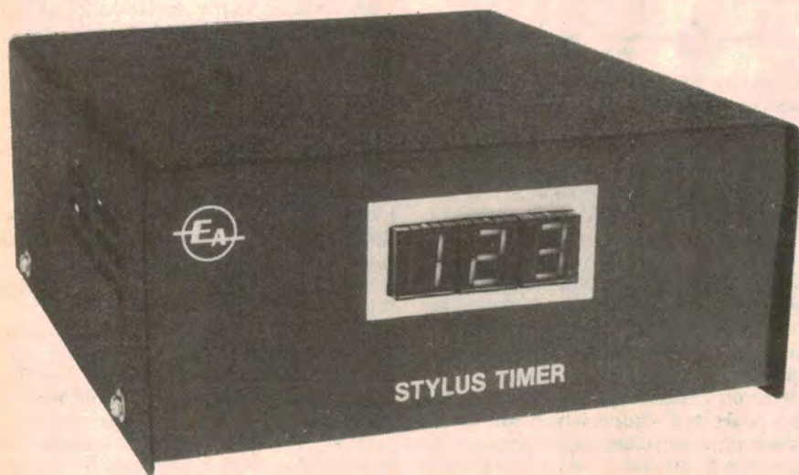
The stylus timer counts the number of hours that the turntable is in use. Standby batteries maintain the count while the turntable is turned off.
