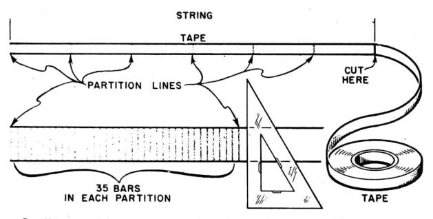
For 331/3-rpm speed there must be exactly 35 equally spaced bars in each of the six partitions.
