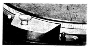
For constant indication of turntable speed, connect a neon lamp to AC line, install near rim.
