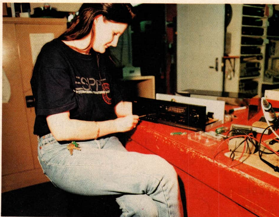
Clare Robbins, a technician at the University of Western Sydney in Kingswood, adjusts the azimuth of a cassette deck. Azimuth adjustment is discussed in the second of these articles.
