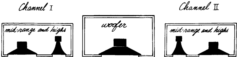
Fig. 122. Putting the woofer in the center gets rid of the apparent dead spot in the middle.
