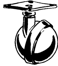
Fig. 528. Casters must be chosen with a view as to how often the cabinet is going to be moved and how much weight it will have to carry. The one illustrated here is a good general purpose type.
