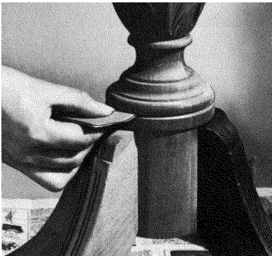
Fig. 703. Curved and carved portions of the cabinet must be finished by hand. Do not use a sanding block. (Courtesy Grand Rapids Varnish Corp.)
