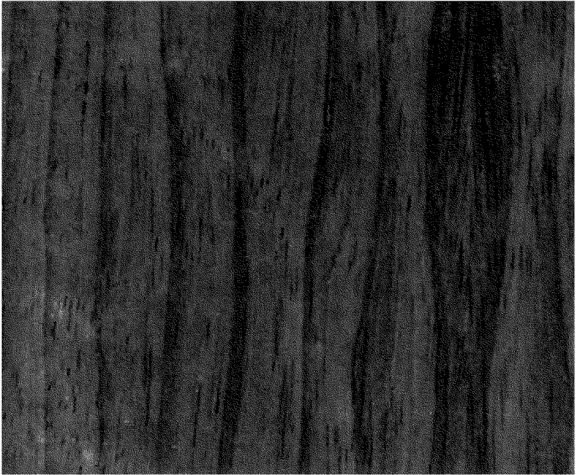
Fig. 510. Blond limba or korina has a grain resembling mahogany and is sometimes sold as bleached mahogany. Also of African origin, it is in wide use. (Courtesy Hardwood Plywood Institute.)
