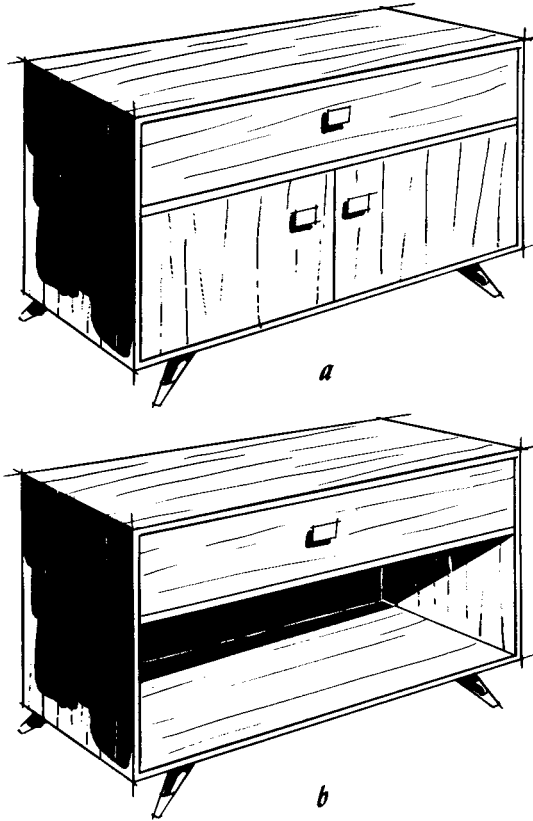
Fig. 331. The use of depth as a dimension: (a) simple drop front cabinet with storage space; (b) removing the lower doors makes the bottom section recede, changing the character of the piece.
