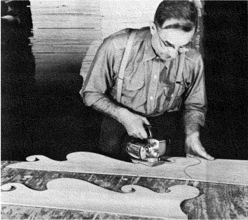
Fig. 607. The sabre saw is another machine which is excellent for cutting curves. (Courtesy Porter-Cable.)
