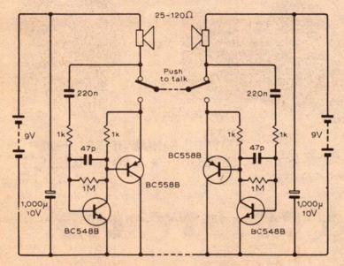
The circuit shows a simple battery powered two-station intercom which does not dissipate any standby power. If NiCd batteries are used, trickle
