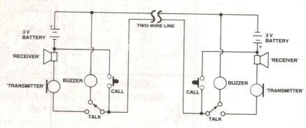
list several suitable types, such as catalogue Nos. 273-004 or 273-060. Pressing either 'call' button will sound both buzzers.
