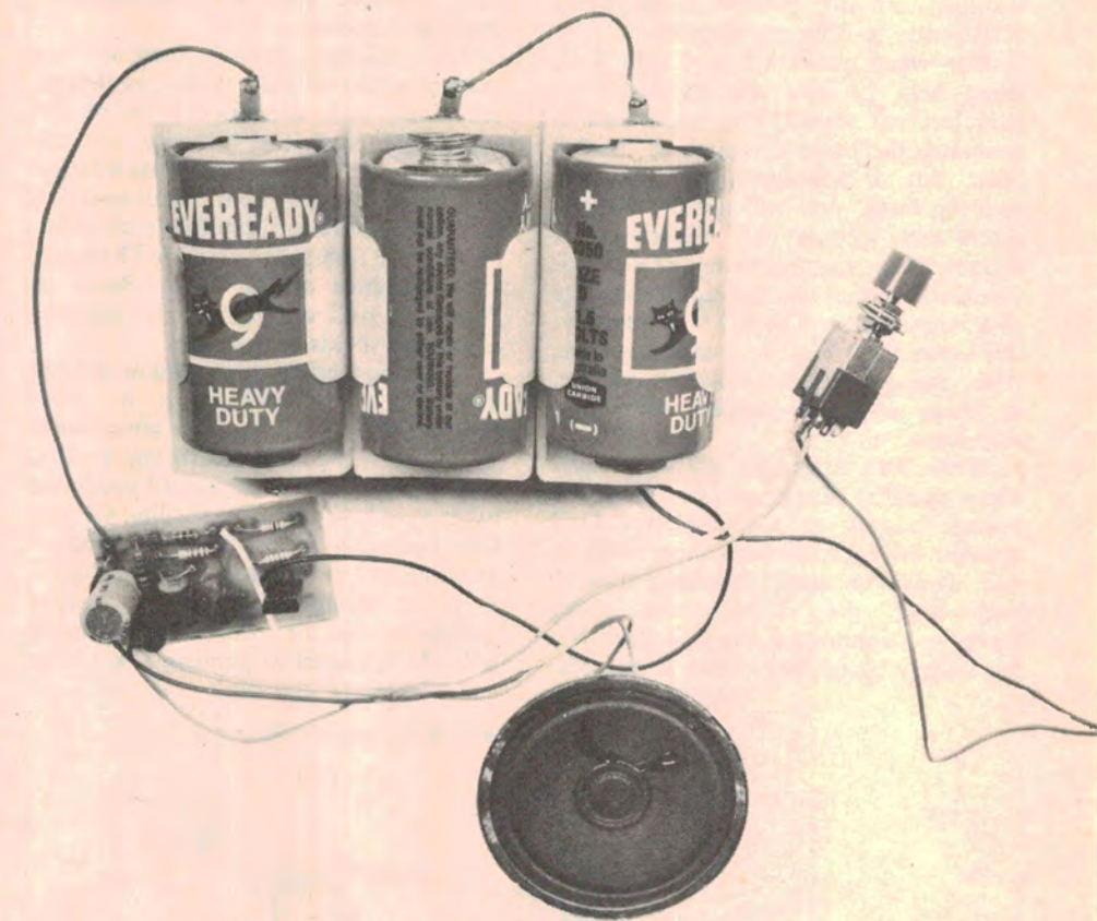
A small loudspeaker serves as both microphone and speaker in this intercom. Housing the project we have left up to you. It is quite possible to fit the components in a palm-sized box, such as one of the small 'zippy' boxes available inexpensively from a number of suppliers. The intercom may be powered from a 3 Vdc plugpack if you wish.
