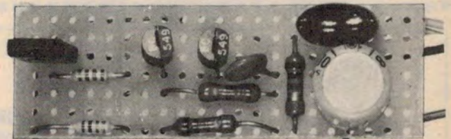
We assembled one unit on a piece of matrix board, laid out as shown.
