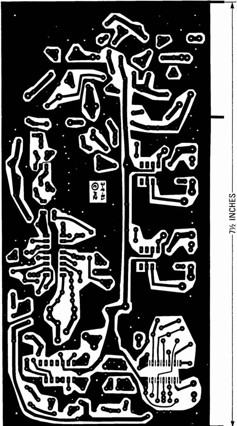
TUNE IN THE HIDDEN WORLD of FM radio with the SCA receiver. Most of the components mount on this single-sided PC board.
