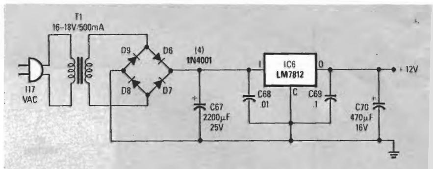
FIG. 3—THE CIRCUIT REQUIRES a regulated 12-volt power supply. The one shown here fills the bill nicely.
