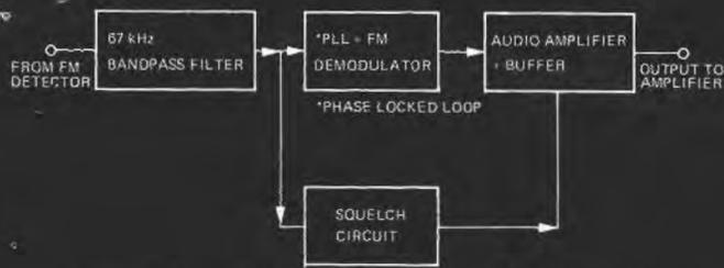
Figure 1 — Block diagram of SCA decoder.
