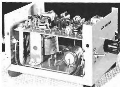
Two views of unit with cover removed showing mounting of decoder and power supply PC boards.
