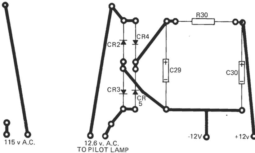
Figure 7 — Printed circuit board for decoder power supply.
