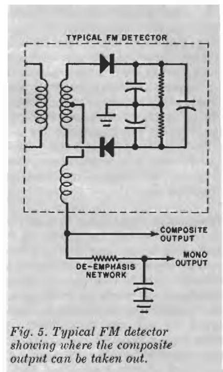
Fig. 5. Typical FM detector showing where the composite output can be taken out.
