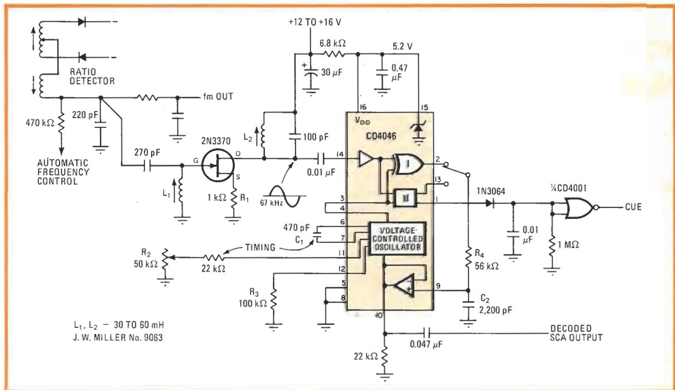
**Simple service.** Improved fm decoder for detecting SCA subcarrier yields higher output, uses fewer parts, provides good selectivity and one option. Requiring only two chips, and one tuned amplifier for separating the stereo from the SCA subcarrier, it costs less than \$10.
