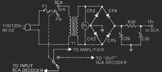
Figure 8 — Optional power supply for SCA decoder.
