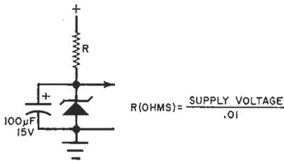
Fig. 4. This circuit is used if you happen to have a vacuum-tube receiver with its high dc voltage. After selecting a 9-to-18-volt zener, and allowing about 10 mA for it, calculate the resistor value.
