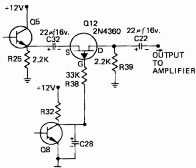
Figure 12 — Schematic for improved muting circuit.
