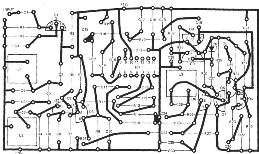
Figure 6 — Printed circuit board for decoder.
