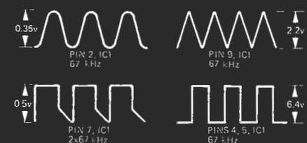
Figure 9 — Waveforms at various pins of IC<sub>1</sub> with SCA signal applied to decoder.
