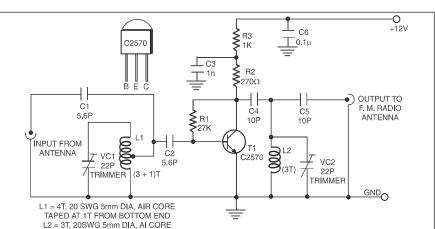
2SC2570. (Only C2570 is annotated on the transistor body.)
