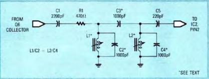
FIG. 1—THIS TUNABLE BANDPASS FILTER effectively suppresses main-channel sputter to provide superior performance for your SCA receiver.
