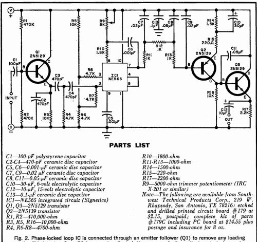
on the FM detector. Once R9 is properly adjusted, there are no further adjustments to be made.
