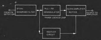
Figure 1 — Block diagram of SCA decoder.
