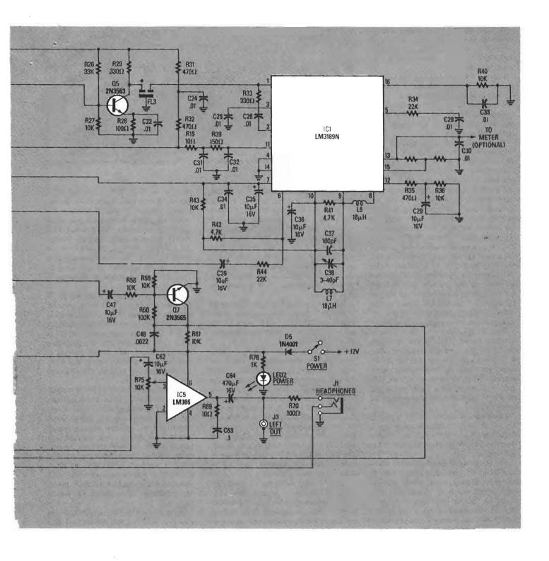
pear at the outputs. Shunt connected capacitors provide de-emphasis. An LED can be connected to the decoder to indicate stereo reception.
