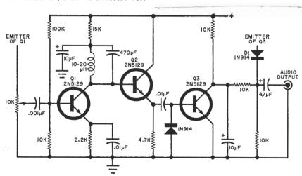
Fig. 1. This squelch circuit can be used with the PLL SCA Adapter to remove the background noise when the SCA carrier is removed during portions of the regular program.
