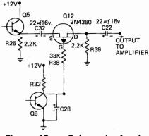
Figure 12 — Schematic for improved muting circuit.
