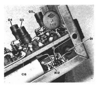
Transistors can be installed in sockets or soldered directly to lugs. Locate a.c. filter capacitors on underside of terminal board and the barrier block at end of box.
