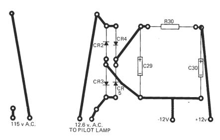
Figure 7 — Printed circuit board for decoder power supply.
