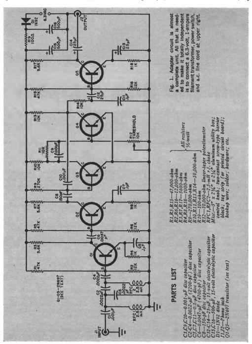
to the point where Q4 is cut off completely all the time. This point is slightly the audio spectrum; therefore, the multivibrator will deliver an output for the full subcarrier modulation range.
