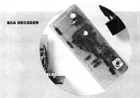
SCA Decoder. Our final PLL project is an SCA decoder built around the 565 phase-locked-loop IC. This is essentially a 67-kHz FM detector. However, a PLL is a better detector for FM than any of the traditional detector de-
