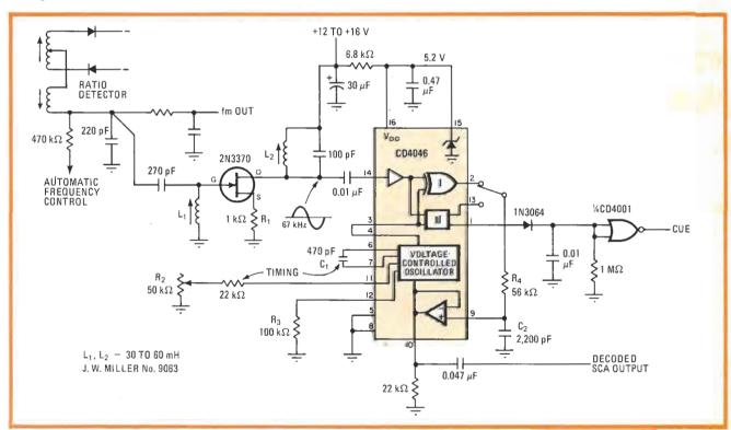
Simple service. Improved fm decoder for detecting SCA subcarrier yields higher output, uses fewer parts, provides good selectivity and oue option. Requiring only two chips, and one tuned amplifier for separating the stereo from the SCA subcarrier, it costs less than \$10.
