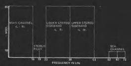
Figure 2 — Frequency allocations within an FM channel.
