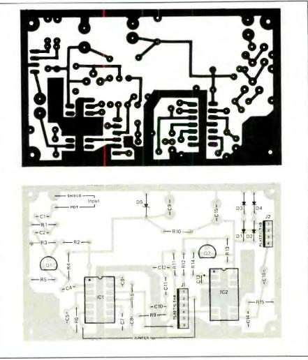
Fig. 3. Shown at the top is the actual-size etching-and-drilling guide to use when fabricating your own printed-circuit board. Install components on this board as shown in placement/orientation diagram at the bottom.
