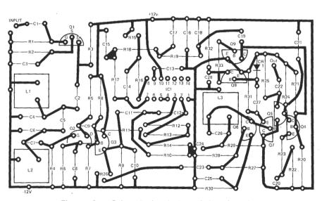
Figure 6 - Printed circuit board for decoder.
