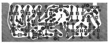
Fig. 3. When installing the components on the board, make sure the IC is oriented properly by noting exactly where the tab is located. Also observe the polarity of the electrolytics and the transistors.
