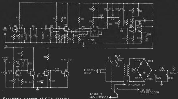
Figure 3 - Schematic diagram of SCA decoder.
