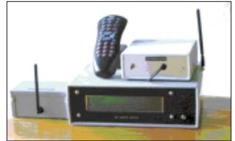
Photo 1: This photo shows the various parts of the system. The mini-box to the left houses the 433-MHz receiver. The case with the large LCD is the MP3 remote control unit. Sitting above it are the RCA remote control and the FM broadcaster module. In normal use, only the FM broadcaster and receiver are located with the host computer, the remote controller is placed wherever you want to listen to the MP3 music.
