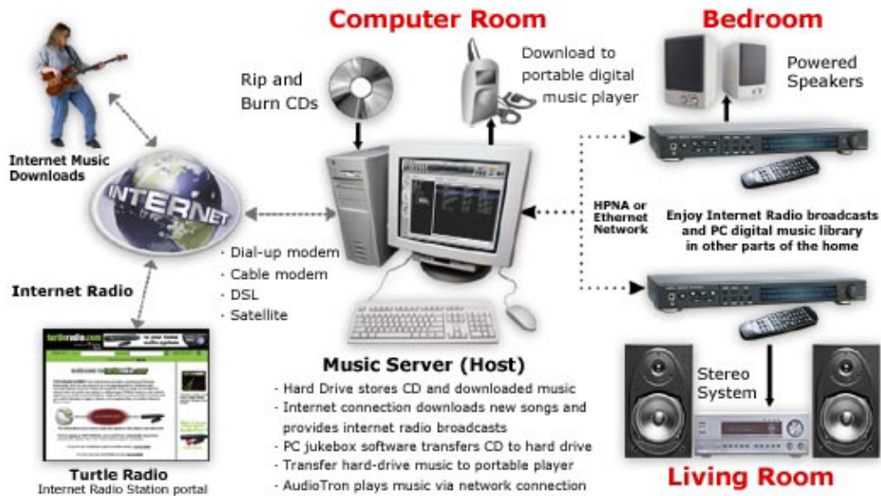
Figure 3 Functional diagram of the AudioTron [3]
