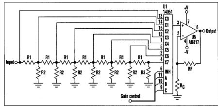
This wide-bandwidth, low-distortion programmable gain amplifier (PGA) is built using low-cost standard devices, eliminating the need for an expensive programmable-gain amp IC.
