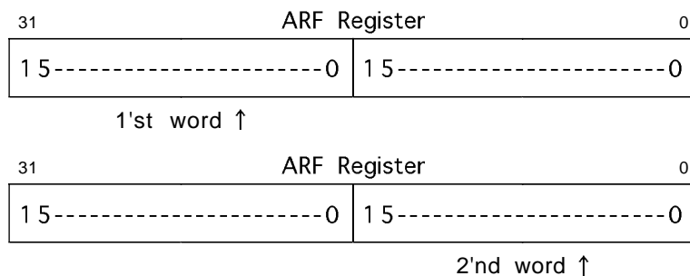
Figure 5-3-11 Register Operation (ARF) for 16-Bit Width DMA Access
