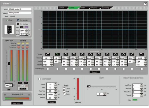
The RHAON Module's DSP is designed for "technical" or "corrective" functions. 8 bands of parametric equalization are available, along with high and low cut filters and high and low shelving filters.
