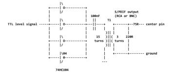
This circuit is part of circuit "Splitter for S/PDIF coax/optical output" by T. Giesberts from Elektor Electronics magazine July/August 1995 pages 78-79. The transformer T1 is made to G2.3-FT12 ferrite ring core. Primary coil is 15 turns of 0.5 mm diameter enamelled copper wire and secondary is 3 turns of 0.5 mm diameter enamelled copper wire. The chip 74HCU04 is manufactured by <u>Philips</u>
