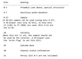
The number of subframes that are used depends on the number of channels that is transmitted. A CD-player uses Channels A and B (left/right) and so each frame contains two subframes. A block contains 192 frames and starts with a preamble "B":
