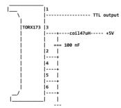
The 47 microhenry coil and 100 nF capacitor make a filter against digital noise in +5V power source. The Toslink receiving module used in this circuit is TORX173 from Toshiba. This circuit is a part of circuit diagram from Elektor Electronics magazine issue 4/1997 page 66.
