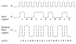
The frequency of the clock if twice the bitrate. Every bit of the original data is represented as two logical states, which, together, form a cell. The length of a cel ('timeslot') is equal to the length of a databit. The logical level at the start of a bit is always inverted to the level at the end of the previous bit. The level at the end of a bit is equal (a 0 transmitted) or inverted (a 1 transmitted) to the start of that bit.
