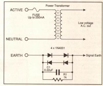
power equipment in a connected group, but retain the proper, solid ground for anything that has a heatsink or fan.
