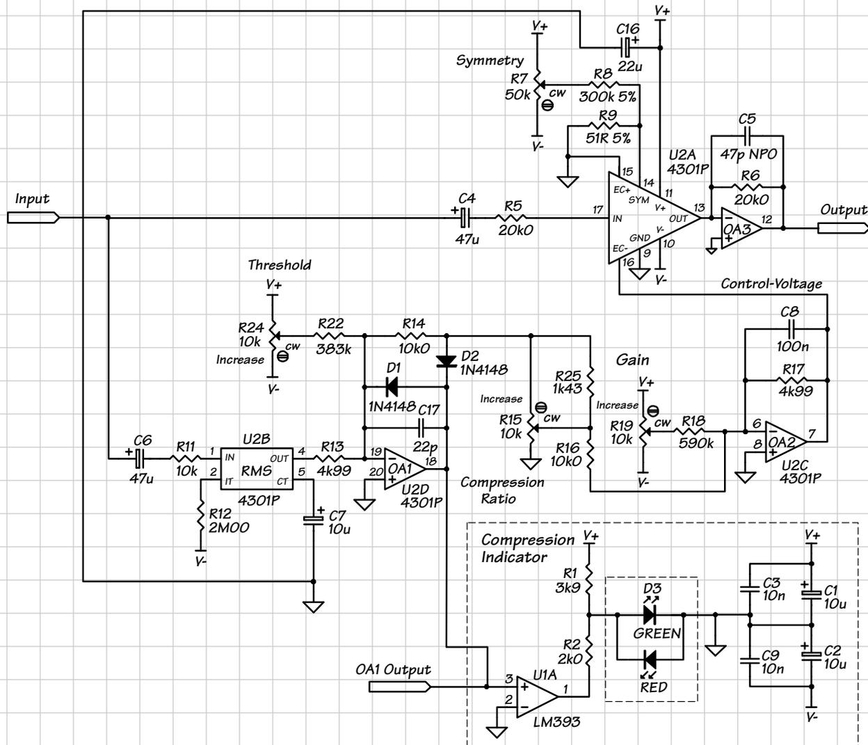
Figure 1. A hard knee compressor/limiter with a bi-color LED to indicate above/below threshold
