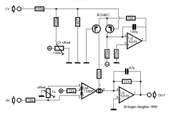
This circuit is identical to LM13600 VCA 1, with the exception of the output stage. Here, the load resistor is in the feedback loop of an inverting amplifier, instead of connected to ground. The effect this has on performance turned out to be neglible. Signal bledthrough seems to be very slightly better, which makes this circuit to the overall winner.
