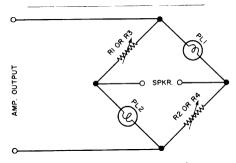
Fig. 1. Basic bridge circuit used.
