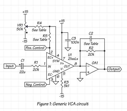
The circuit in Figure 1 shows a generic VCA circuit that can be adapted for use with all of THAT Corporation's standalone VCAs by the inclusion or omission of different values of components. This circuit allows complementary drive of both control ports, but unidirectional (single-ended) drive of either control port can be achieved by grounding the undriven port. 1
