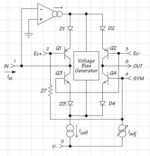
Figure 2: Simplified Internal Circuit Diagram
