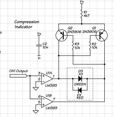
Figure 3. Compression indicator with no ground current and optimal LED drive
