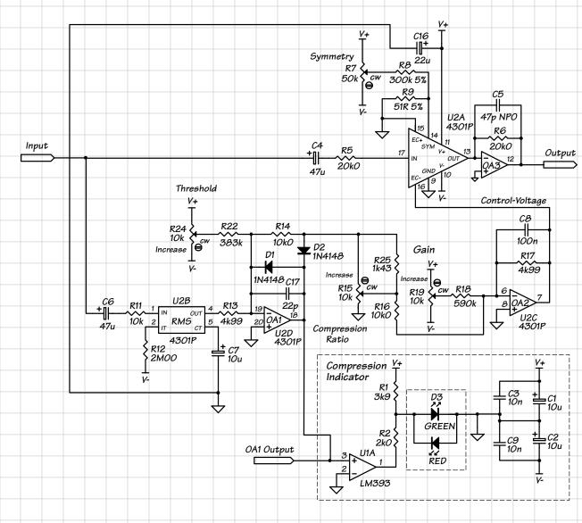
Figure 1. A hard knee compressor/limiter with a bi-color LED to indicate above/below threshold
