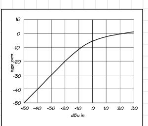
Figure 8. Soft knee threshold characteristic
