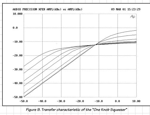
During normal operation, the user should adjust the gain of the signal chain ahead of the compressor so that the average signal level is at the desired nominal listening level (in this case, -10 dBu). Once this level is set, the user can easily add compression with a single adjustment, backing off when pumping or sibilants become noticeable or the signal sounds overly compressed, all without the distraction or confusion caused by changes in output level.
