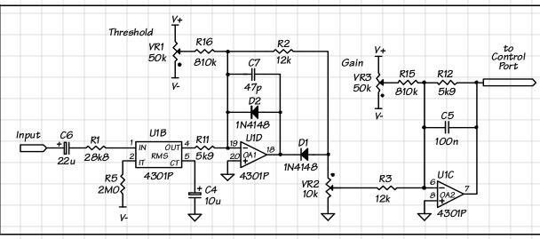
Figure 1. Basic comp/limiter sidechain with independent gain and threshold
