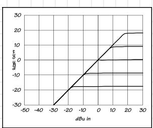
Figure 2. Typical hard knee threshold characteristic
