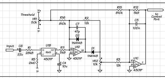
Figure 5. Comp/limiter sidechain with complementary gain and threshold
