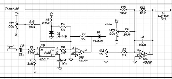
Figure 7. Soft knee comp/limiter with complementary gain and threshold
