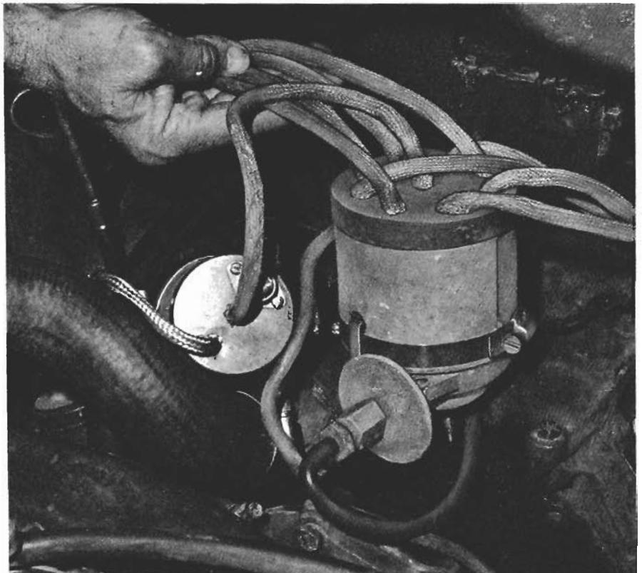
At center is the distributor with a shield can clamped over it. In the technician's hand are high-tension wires encased in shield braid.
