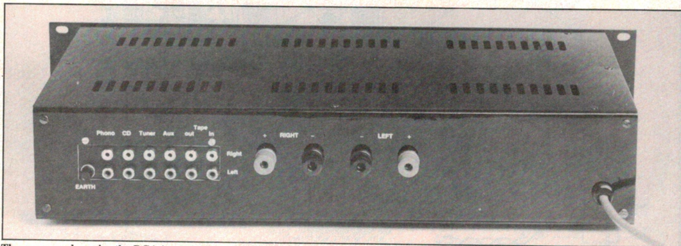
The rear panel carries the RCA input sockets and the loudspeaker terminals. Make sure that the mains cord is securely clamped.
