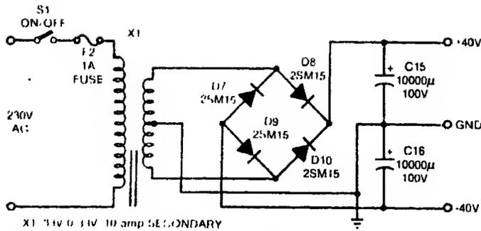
Fig. 4: Suggested power supply for the circuit.
