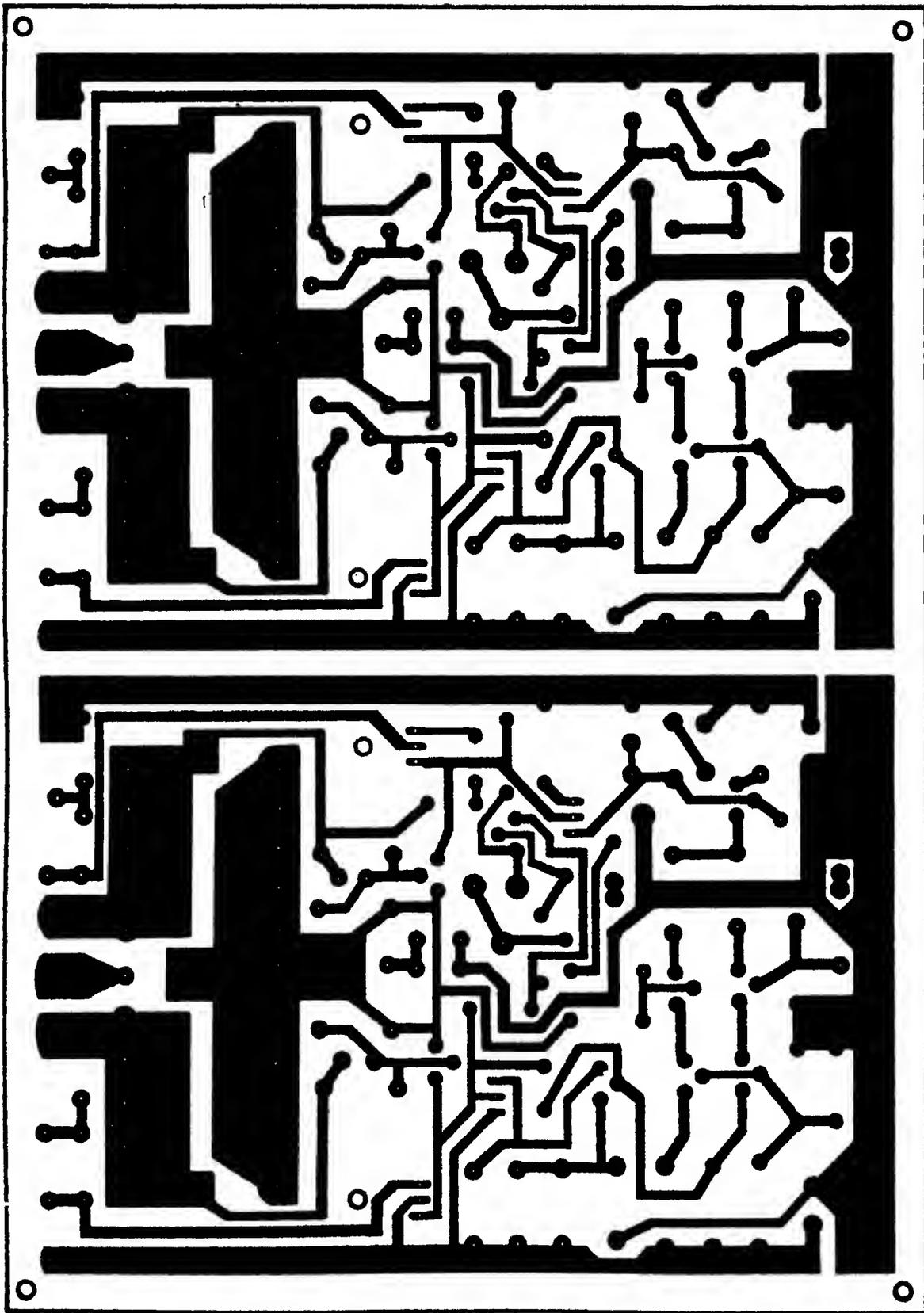
Fig. 2: PCB layout for 120W + 120W stereo amplifier.
