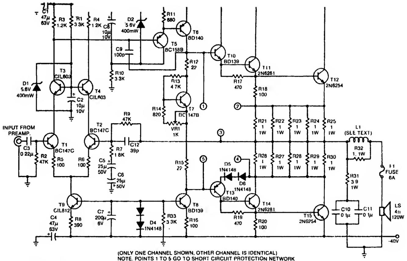
Fig. 1: Circuit diagram for 120W + 120W stereo amplifier.
